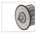
If the blind does not reach, you can turn the wheel the opposite way to extend the pin out further, and again for a second time if needed. This is handy if there has been a slight mismeasure.
